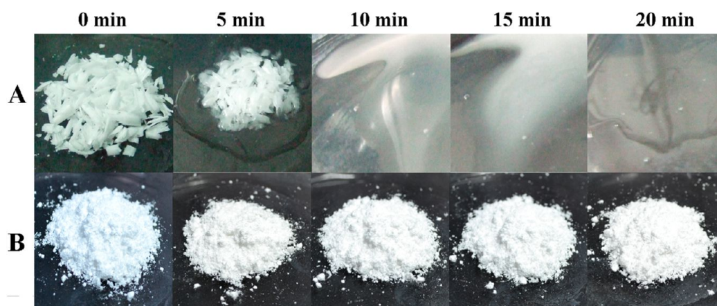
Figure 7. Photographs of pure paraffin (row A) and paraffin@SiO 2 composite (row B) heated at 70 °C for different times.
